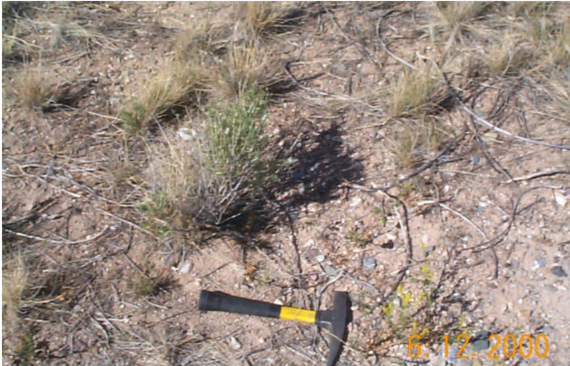
Photo 37: Close-up of the surface of the “typical” test plot on the surface of a tailings area covered and revegetated in 1993 (Dam 1 tailings area).
