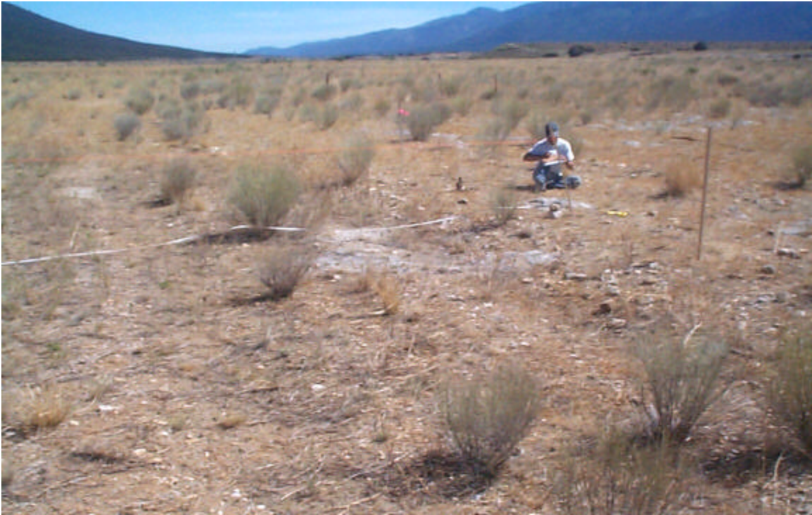
Photo 41: The 30 ft x 30 ft test plot representative of “more erosive” conditions on the surface of a tailings area covered and revegetated in 1993 (Dam 4 tailings area).
