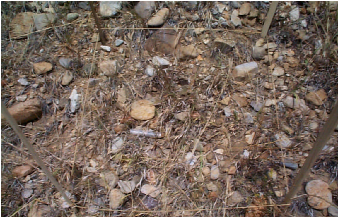
Photo 3: A 3 ft x 3 ft test plot created on the lower slope of Dam 1; representative only of the coarse rock (i.e. not vegetation) on the dam slope.
