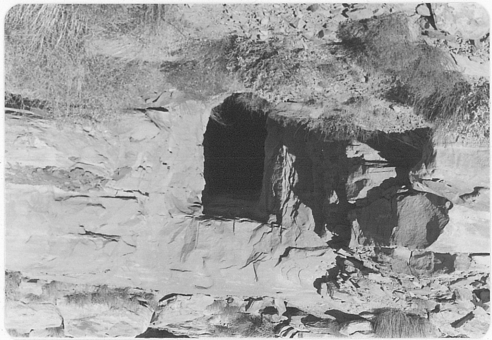
Photo (c) Close-up of north trending adit from which waste dump shown in photo b was produced; portal is approx. 6' x 3', adit is at least 50 long. Scintillometer readings averaged 100 cps (or 2x background).
