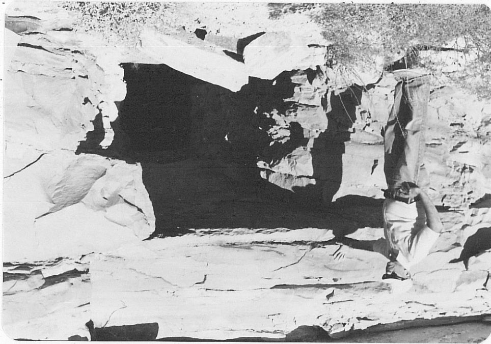
Photo (c) Close-up of north trending adit from which waste dump shown in photo b was produced; portal is approx. 6' x 3', adit is at least 50 long. Scintillometer readings averaged 100 cps (or 2x background).
