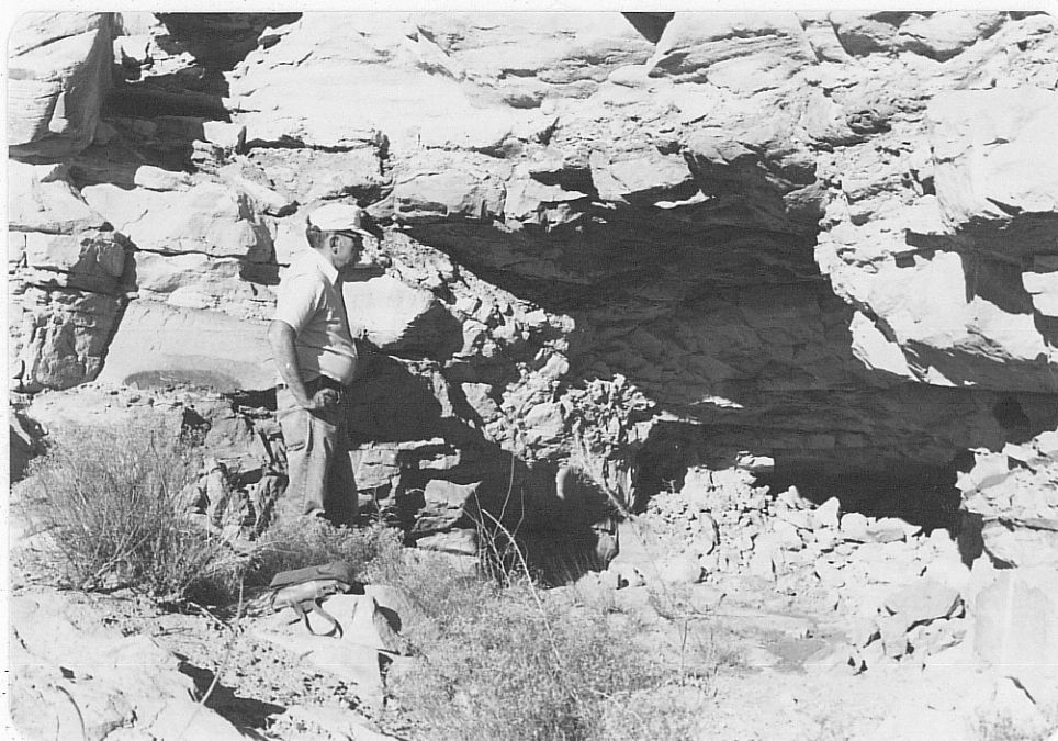
Photo (f) Close-up of adit shown in photo e; opening is 6' high, 8' wide and 10' long; heading nearly due north; maximum scintillometer readings of 1700 cps were obtained. Locale is near southeast corner of claim.
