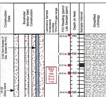
157.5'-158.5' Split Spoon 0.8' sample. Entire core is (SM) light brown yellow (10YR) very fine sand with trace silt and fine sand, unconsolidated, slightly moist, no apparent hydrocarbon odor in cuttings.
