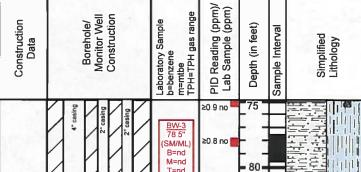
77.5'-79.5' Split Spoon 2.0' sample. (SM/ML) (10YR) Light brown to tan silt to very fine sand, slightly moist to moist, unconsolidated, no apparent hydrocarbon odor in cuttings, massive, no bedding, only trace calcium carbonate.
