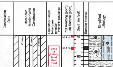
77.5'-78.7' Split Spoon 1.2' sample. (SM/ML) (7.5YR) Reddish yellow silty very fine sand, unconsolidated sand for ~5-10% calcium carbonate cemented nodules, slightly moist, no apparent hydrocarbon odor in cuttings.
