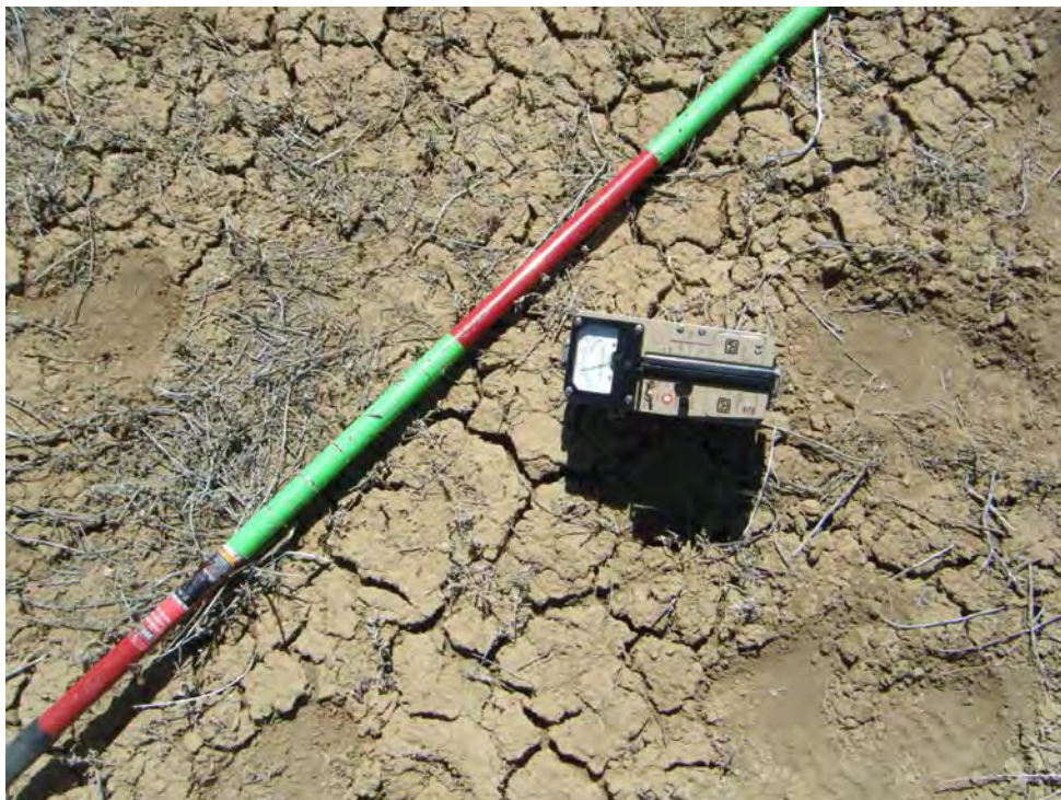
Photo 4-Radiation survey point Rad-3 (150 \mu R/hr at 0 meters).
