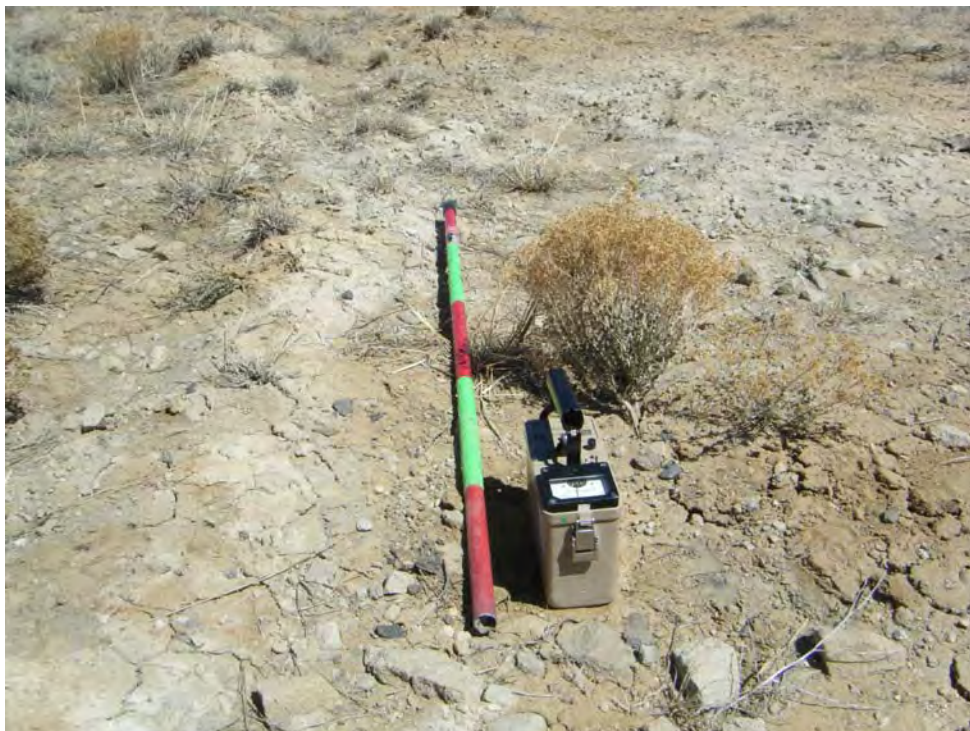
Photo 8-Radiation survey point Rad-6 (350 \mu R/hr at 0 meters).
