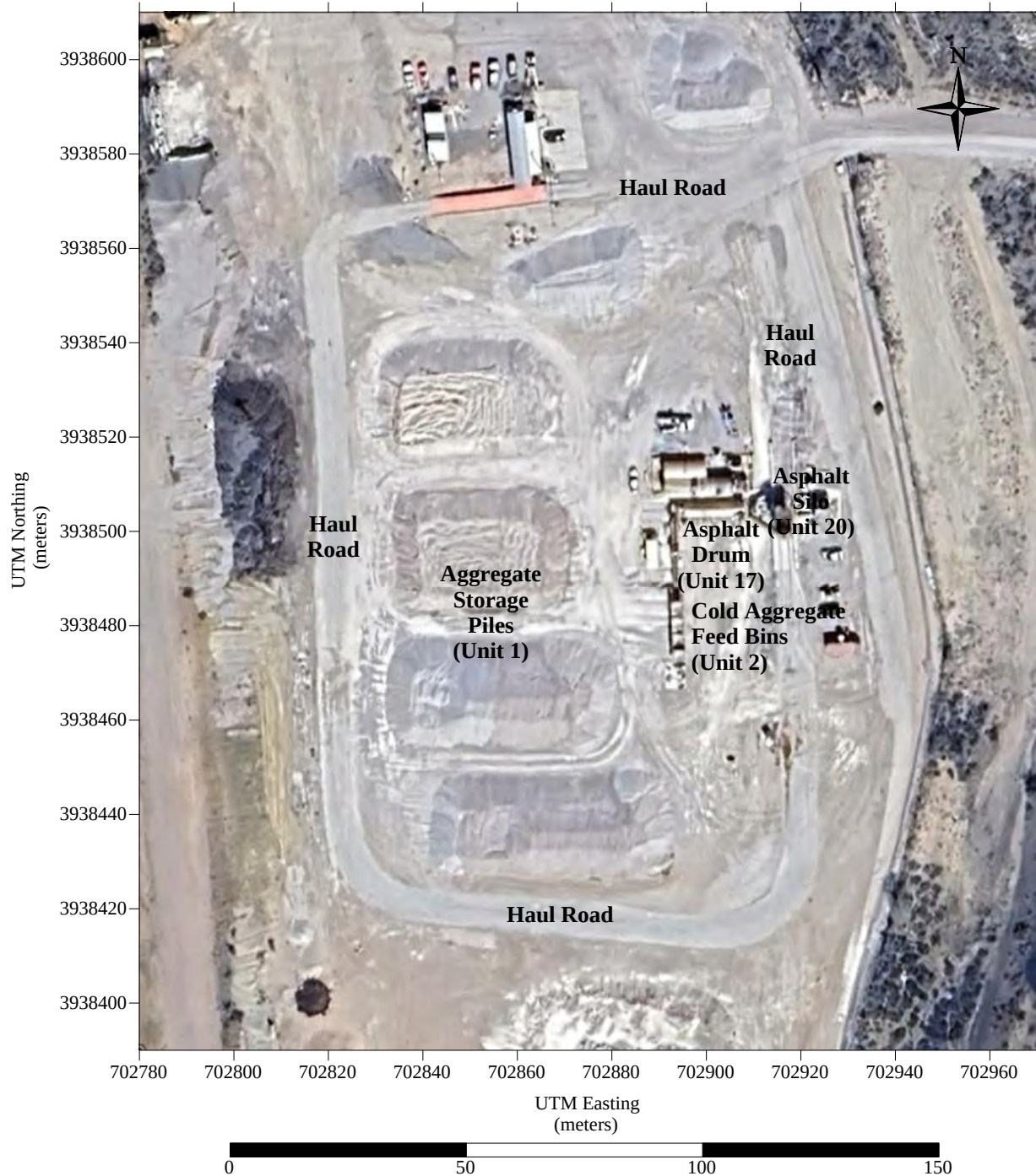
Figure 5-1: HMA Plant Site Layout
