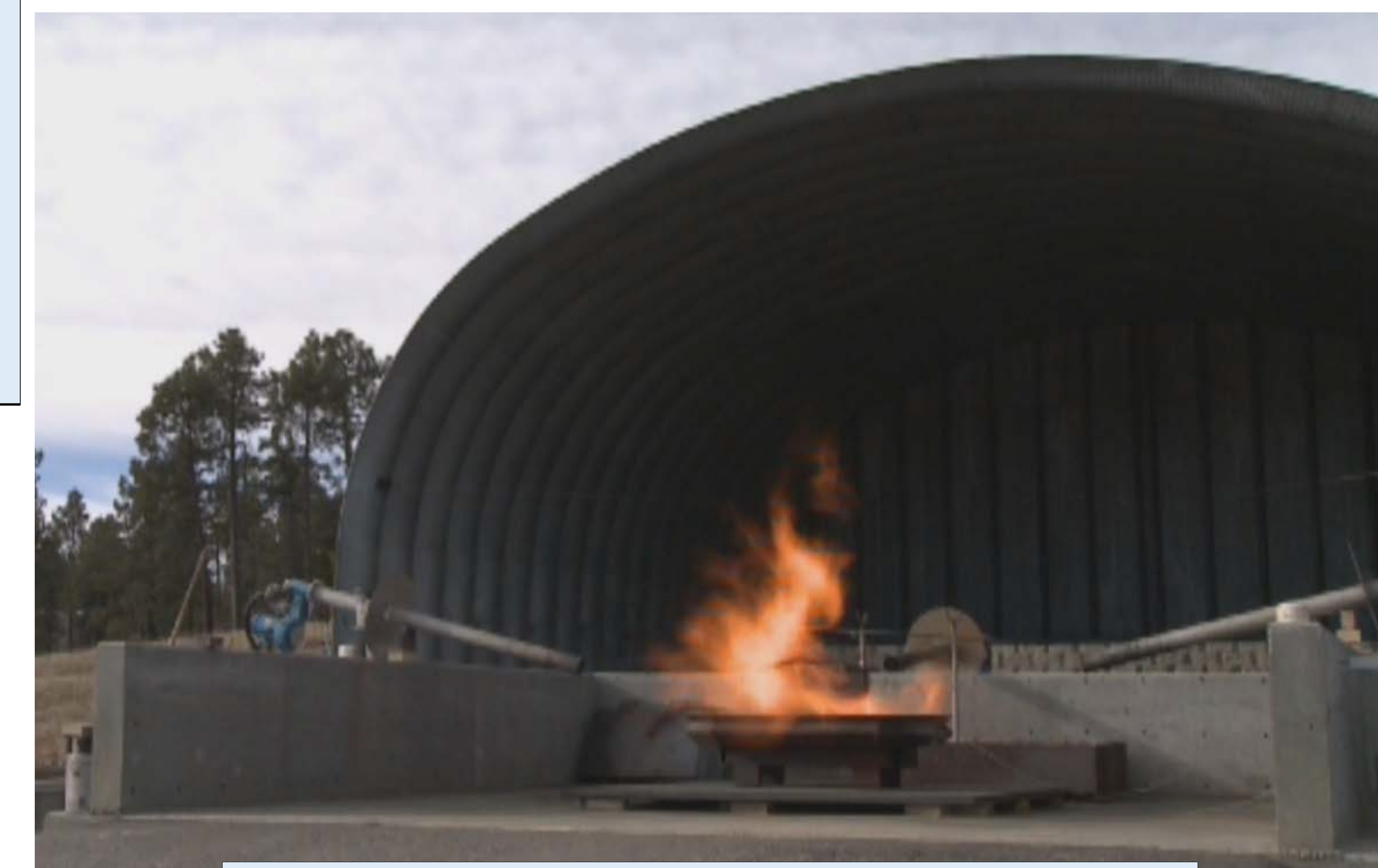
TA-16-388 Flash Pad Unit in use and uncovered, left burner igniting
