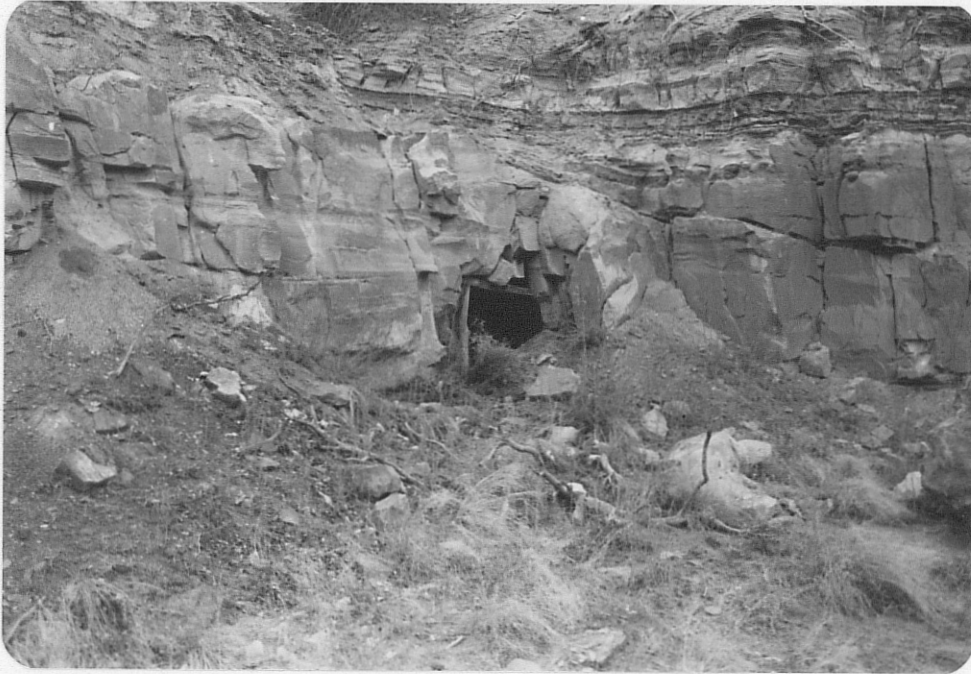
Photo (c) Adit in Salt Wash member, thought to be on Joe Ben #3 claim; looking westward. Note field glasses hanging above adit entrance for scale; also note scour and fill feature above and to right of adit.
