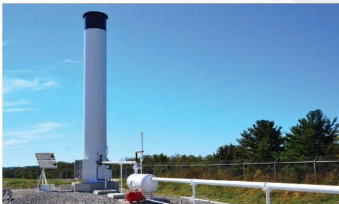
ZEECO® Engineered Enclosed Flare System
