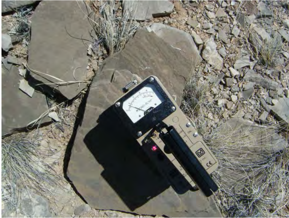
Photo 5-Radiation survey point Rad-9, taken on Todilto Limestone, measuring 100 \mu R/hr at contact.
