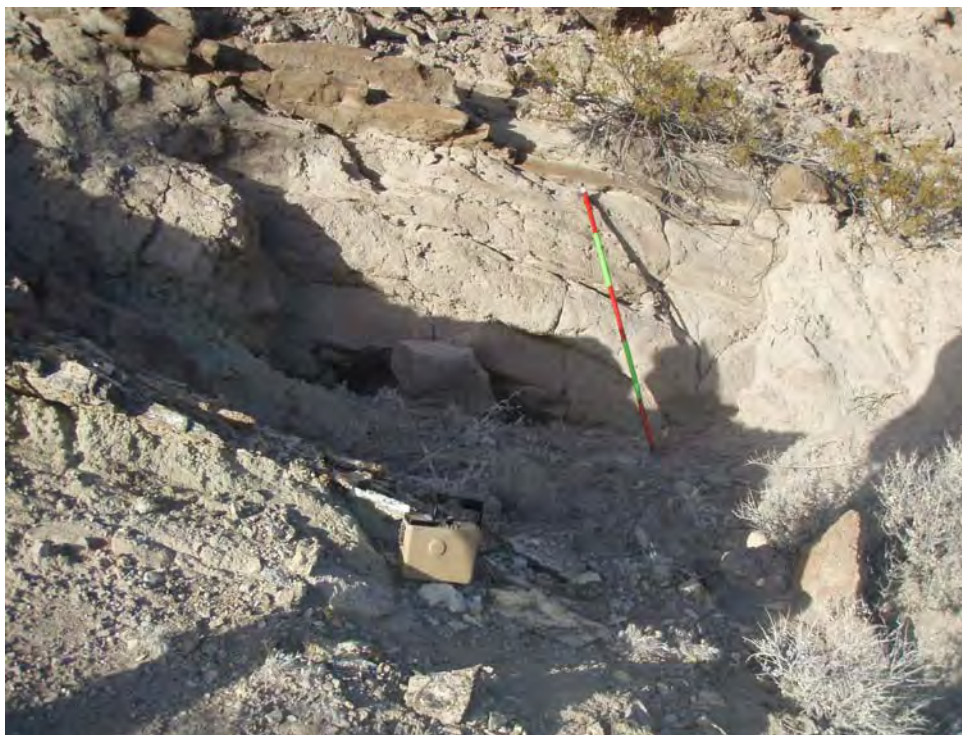
Photo 28 - A small exploration pit (pit-2) near the Cabra Canyon road. The scintillometer rests on the Uranium bearing tuffaceous sandstone.
