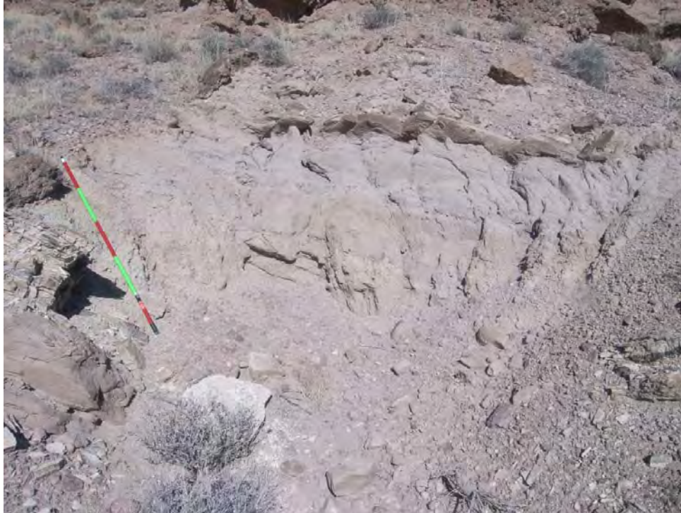
Photo 6 - A shallow prospect pit (pit-1). The uranium bearing formation is just left of the scale pole.
