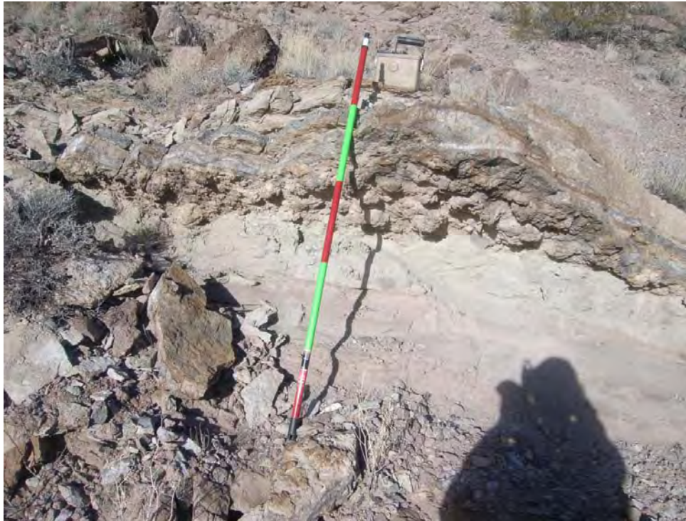
Photo 19 - A uranium bearing layer lies immediately above a weather resistant chert layer, which juts out from the hillside.
