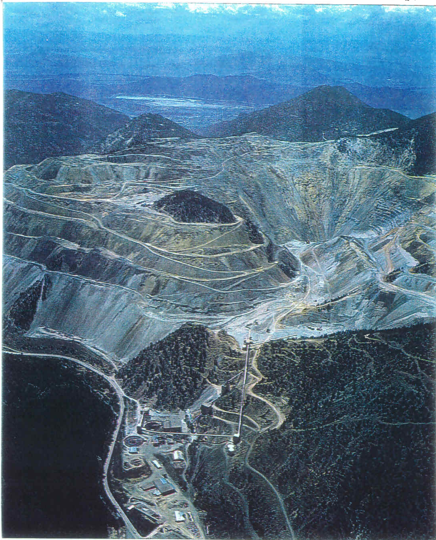
Aerial view of the Molybdenum Questa Mine, showing open pit (right), waste-rock dumps (left), mill facilities (bottom), and tailings impoundments ten miles distant at Questa (light-colored area at top center). The Red River, barely visible in this photograph, flows parallel to Highway 38 in lower left of picture. View is to the west. Photograph by LightHawk, Santa Fe, New Mexico.
