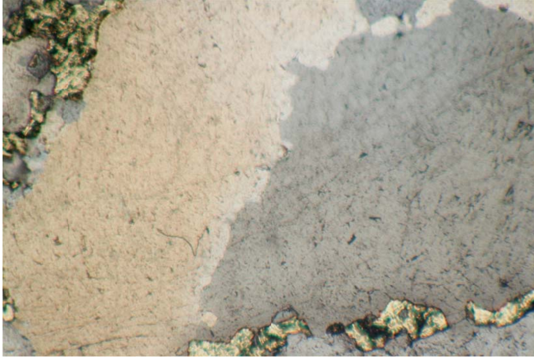
Figure 13-1: Chalcopyrite mineralisation along edges of quartz grains. (XPL and reflected light at x 4 magnification. Field of view = 2.8 mm)
