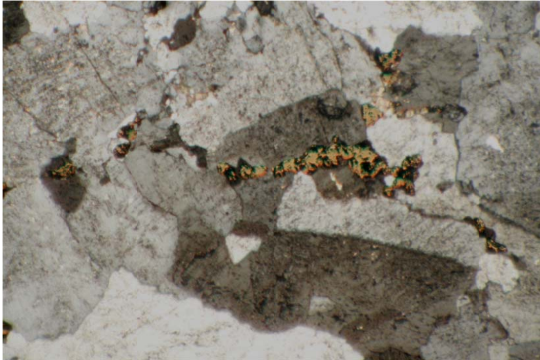
Figure 12-1: Chalcopyrite mineralisation along edges of quartz grains. (XPL and reflected light at x 4 magnification. Field of view = 2.8 mm)
