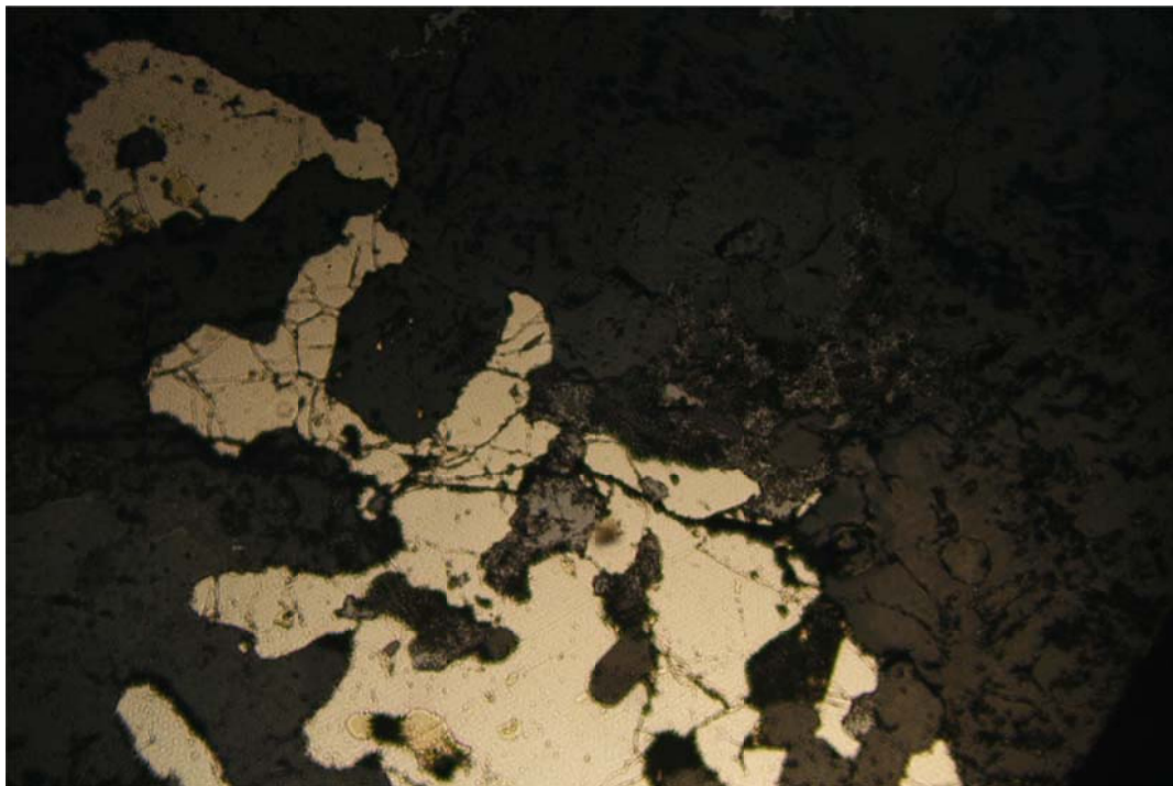
Figure 16-2: Chalcopyrite with quartz. (reflected light at x 10 magnification. Field of view = 1.16 mm)
