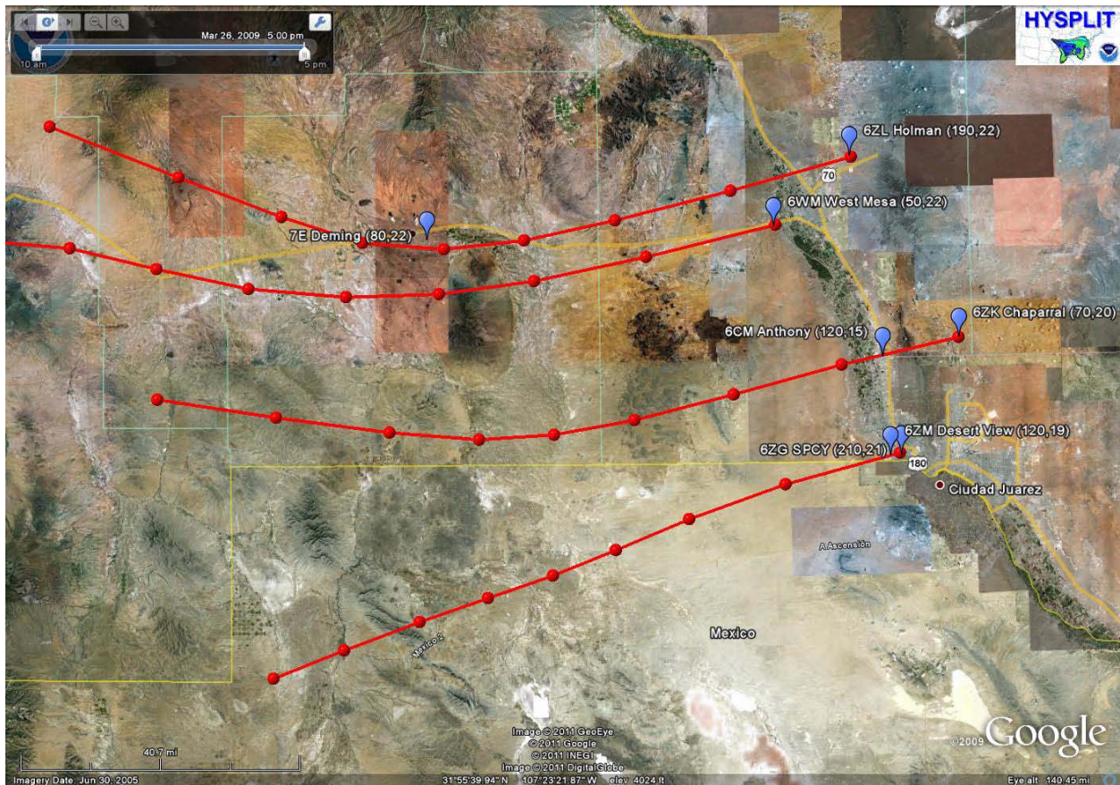
Figure 7-5. Back-trajectory model analysis for the event on March 26, 2009. The numbers in parenthesis are the 24-hour average PM_{10} concentration and max wind gust respectively. The model was run for the eight hours preceding the peak concentrations of the event starting from the 1200 hour. Each ball represents one hour in the past from the starting point of the model run.
