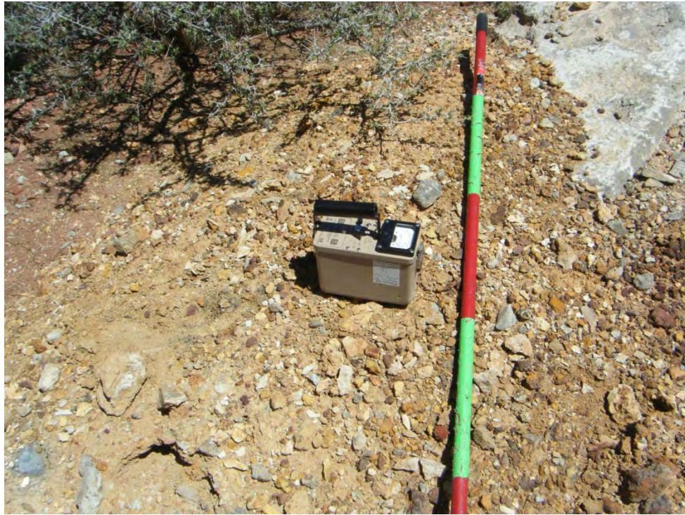
Photo 14-Looking north at radiation survey point Rad-9 (900 \mu R/hr at 0 ft above ground).
