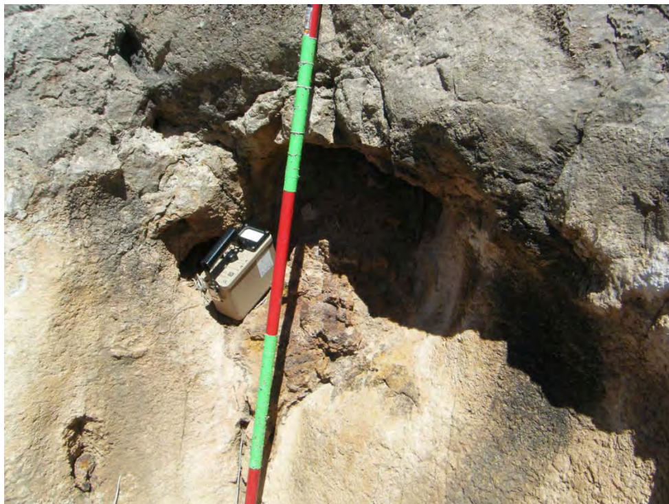
Photo 9-Looking north at radiation survey point Rad-4 (470 \mu R/hr at 0 ft above ground).
