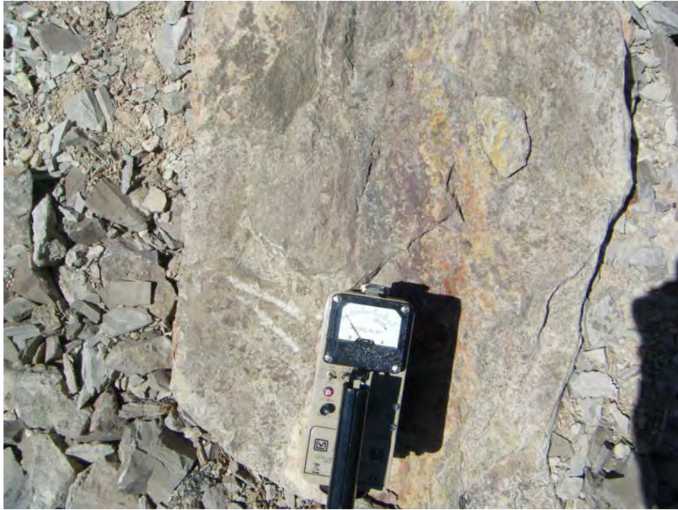
Photo 1-Radiation survey point 1 (800 \mu R/hr at contact; Red Bluff No. 5 claim).
