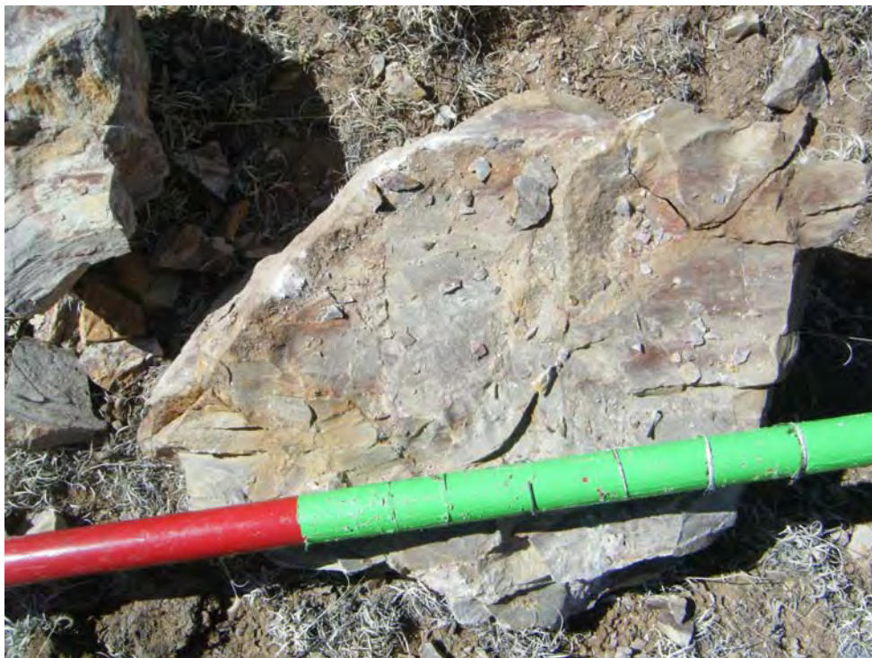
Photo 16-Radiation survey point Rad-7 (1250 \mu R/hr at contact; Red Bluff No. 3 claim).
