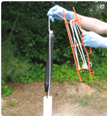
Figure 7 – Example passive diffusion sampler.
