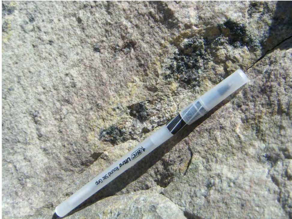
Photo 33-Uranium mineralization at radiation survey point Rad-19 (gamma radiation off scale at >5000 \mu R/hr at contact).
