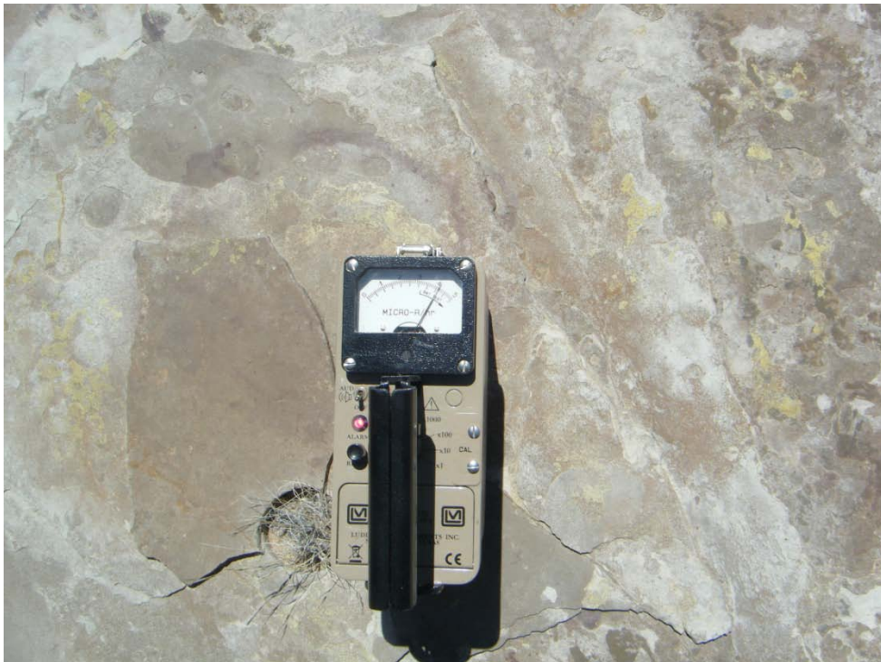
Photo 28-Radiation survey point Rad-17 (4400 \mu R/hr at 0 ft above ground).
