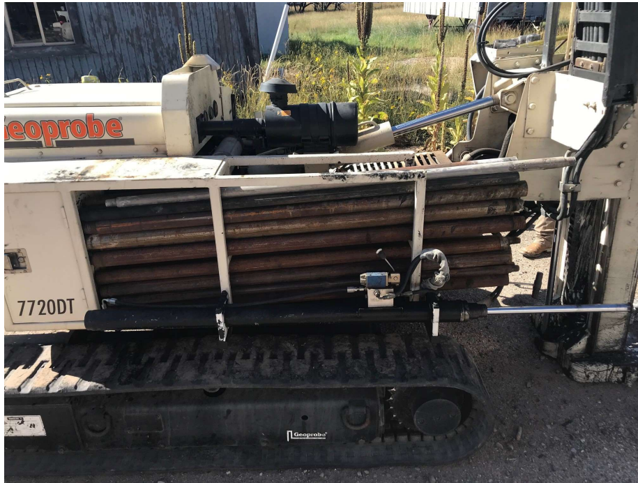
Geoprobe 7720DT Direct Push Rig
