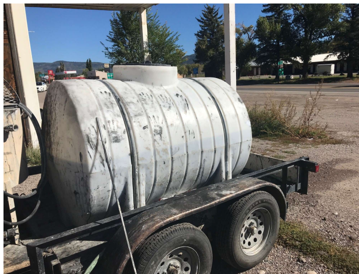
A 500-gallon Water Holding Tank
