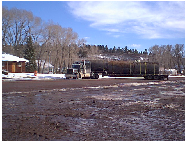
Photo 12: Trucking of USTs.
