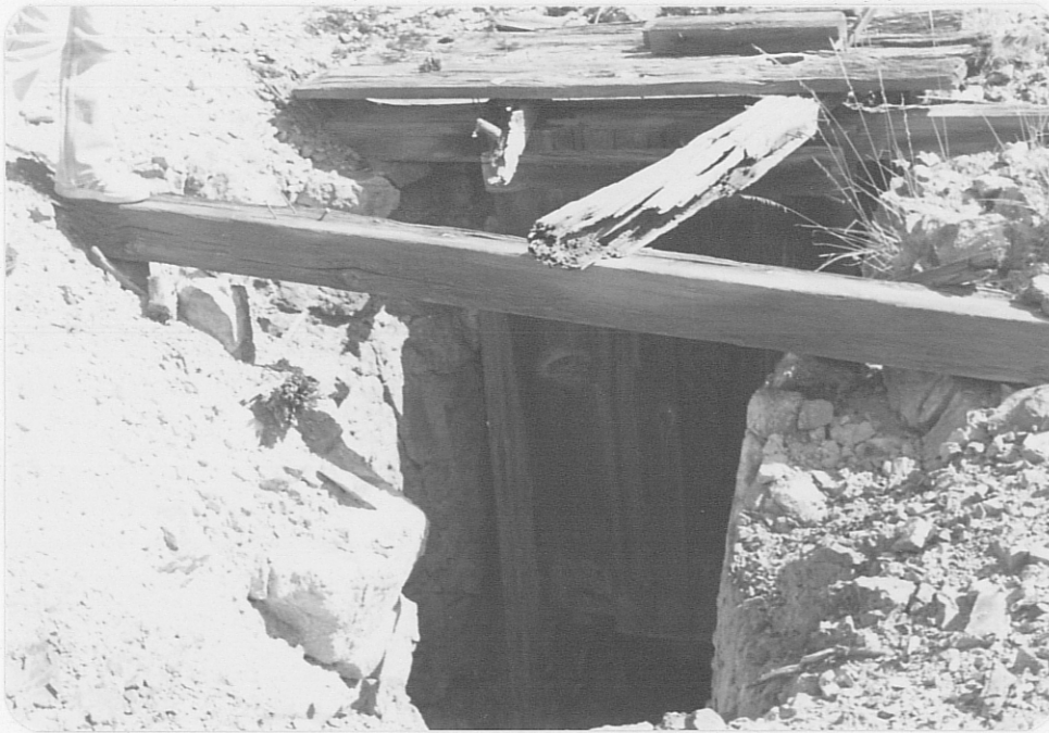
Photo (a) Looking north into covered inclined shaft thought to be on Blue Jay Claims.
