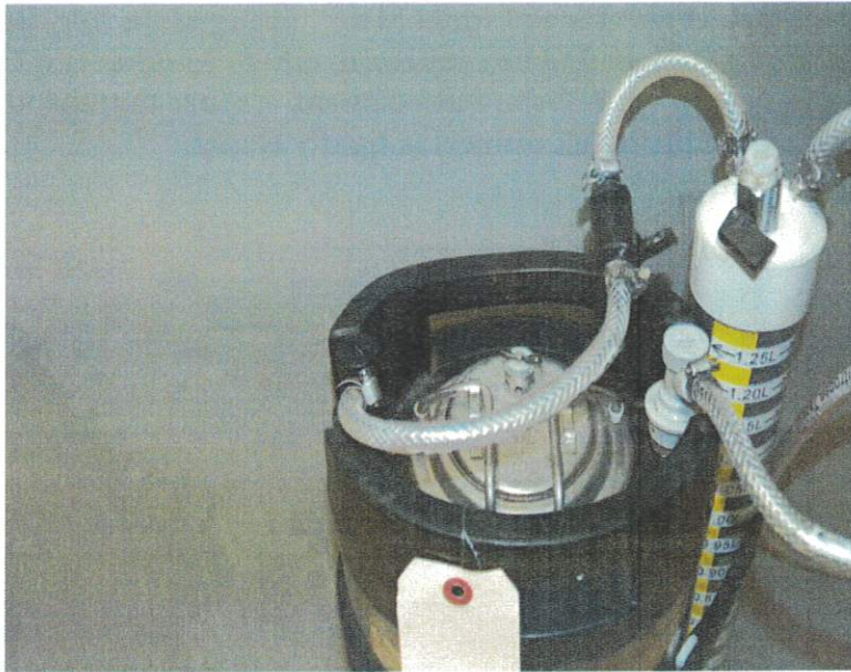
Keg and measuring cylinder attached to the keg's fittings black and grey connectors.
