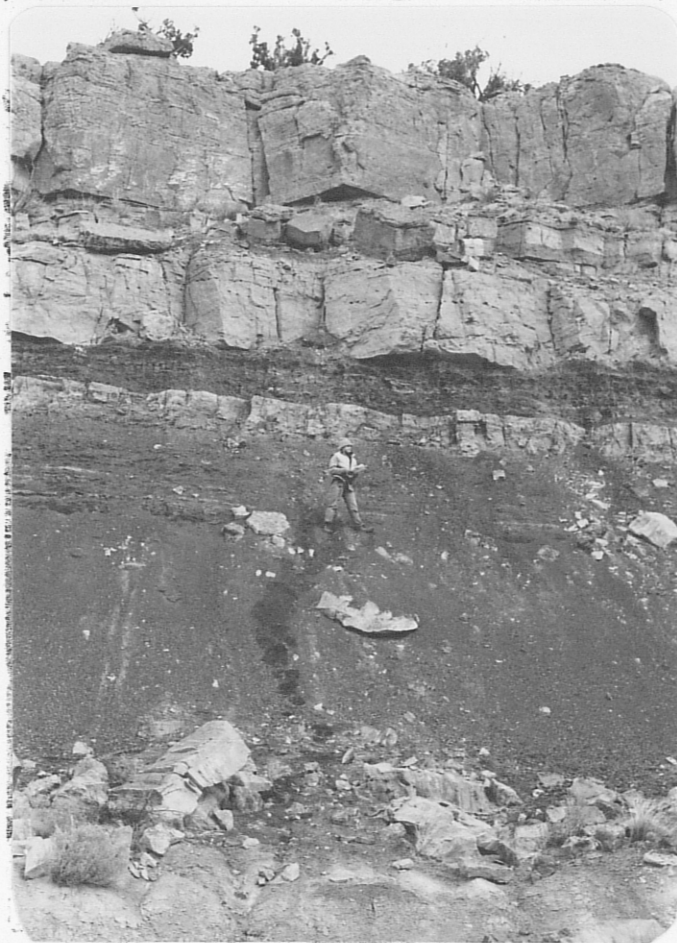
Photo (b) View northward showing a 15' thick sequence of carbonaceous shale just above floor of cut.
