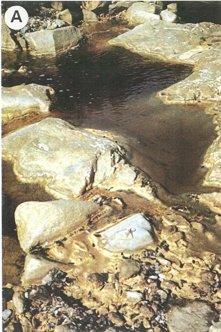
Plate 2. A. Jarosite (yellow) precipitation from an acid mine water (pH 2) in Shasta Co., California. Grey color on stream bed is a coating of bacterial slime. Scale is provided by a ring of keys in center foreground. (See Chapter 3). Plate 2. B. Face of lignite surface mine showing oxidized (about upper 1/5 of exposed soil-geologic column) and reduced zones of the pre-mining column. (See Chapter 10).
