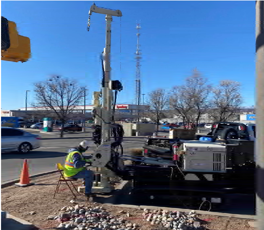
Photo 7 – Soil sampling MW-25 bore hole.
