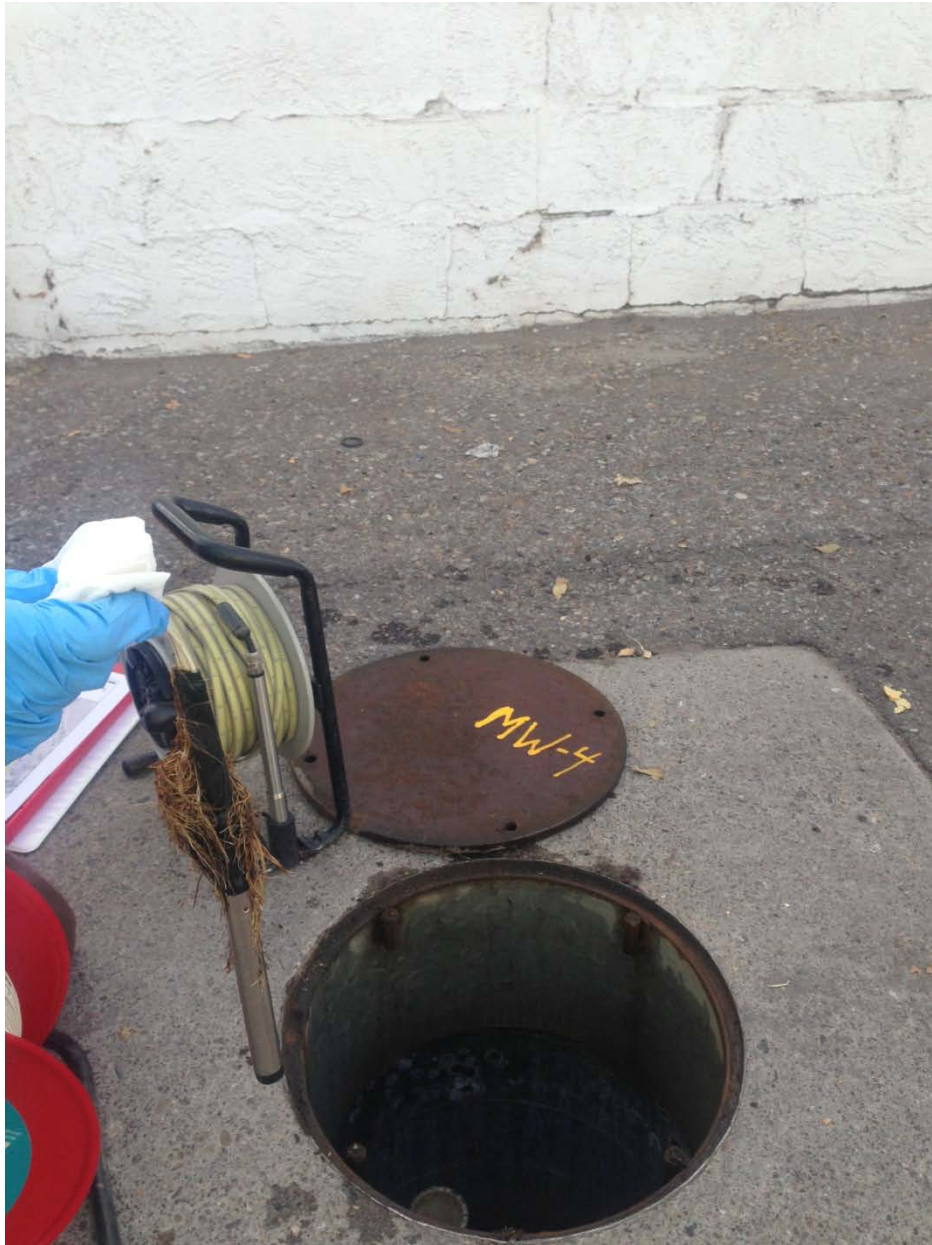
Rootball recovered on oil/water interface probe during fluid level gauging activities at MW-4.
