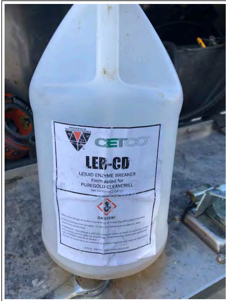
25. Liquid enzyme breaking solution for use during development jetting
