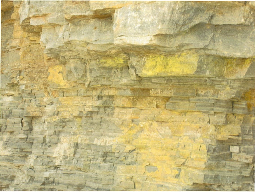
Exposed face of the mine with yellowing on the rocks from exposed areas of uranium. Ludlum reading in this area was over 600,000 cpm. Photo taken March 2011, by LaDonna Turner, EPA.
