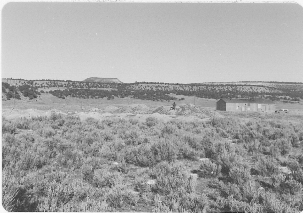
Photo (b) Looking east toward Black Jack #2 tailings dump; dump is more than 300' long, up to 10' high; note person with range pole for scale.
