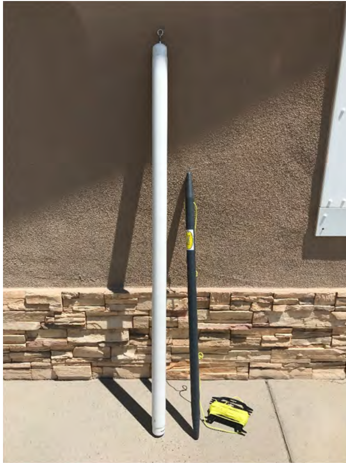
Photo 1: 1.2 and 0.33 gallon slugs for 4 and 2 inch diameter wells
