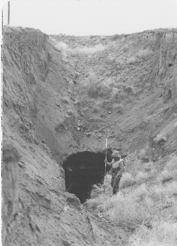
Photo (b) Looking southward at portal of inclined shaft in bottom of box cut.
