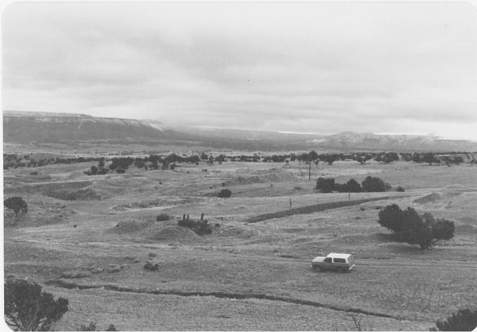
Photo (a) Looking southeastward at the Hanosh shaft site showing load out facility at lower left, and box cut immediately to right which contains entrance to shaft. In background at center and left is spoil piles from strip mining in section 25.
