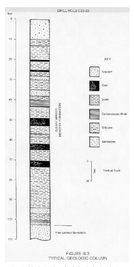
PEABODY EXHIBIT 19. Typical Geologic Column for shallow bedrock within LRM Permit 19-2P.
