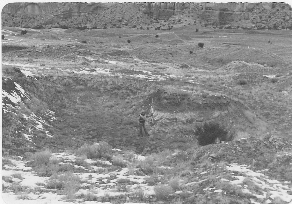
Photo (a) Looking NW into stripped area from SE edge of sec. 24 mine; note overburden piles at upper center and upper left extending for nearly 1,000' away from viewer. Mine trends NW.
