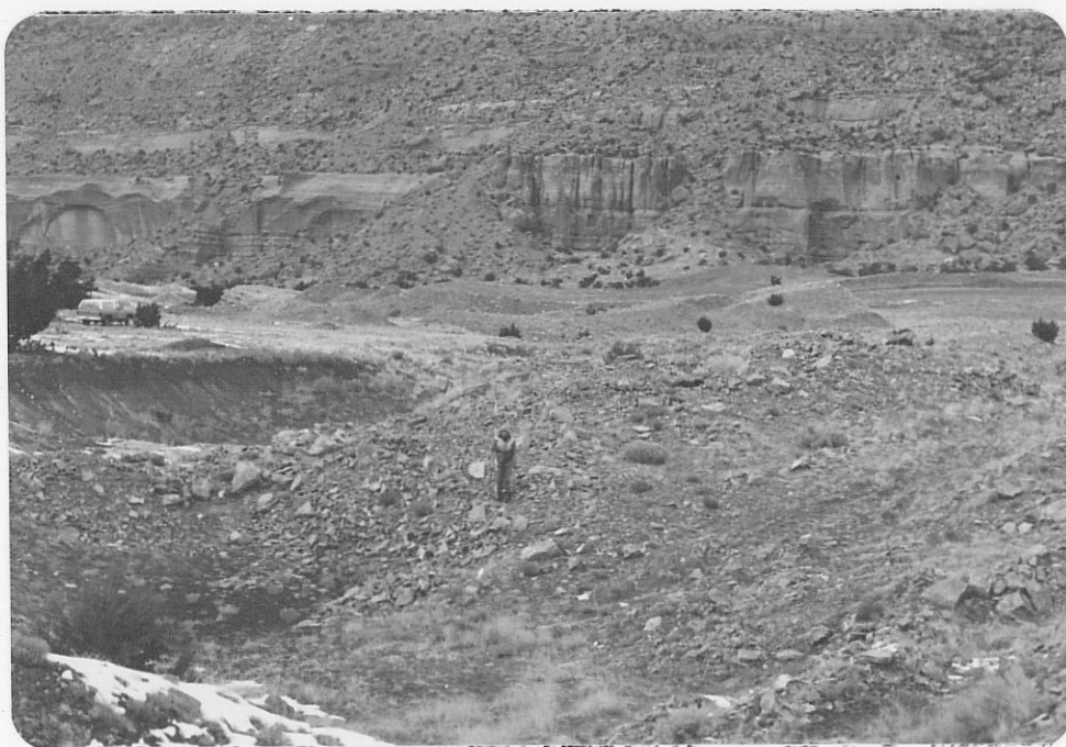
Photo (b) Looking again to NW, from within mine area, showing size and nature of individual pits; unconsolidated overburden is often more than 10' thick as seen in highwall below vehicle at left. Note large overburden and waste piles at center, middle distance.
