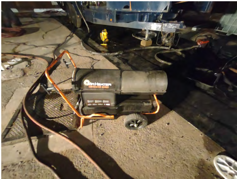
Diesel Heater to Keep PetroFix® Warm
