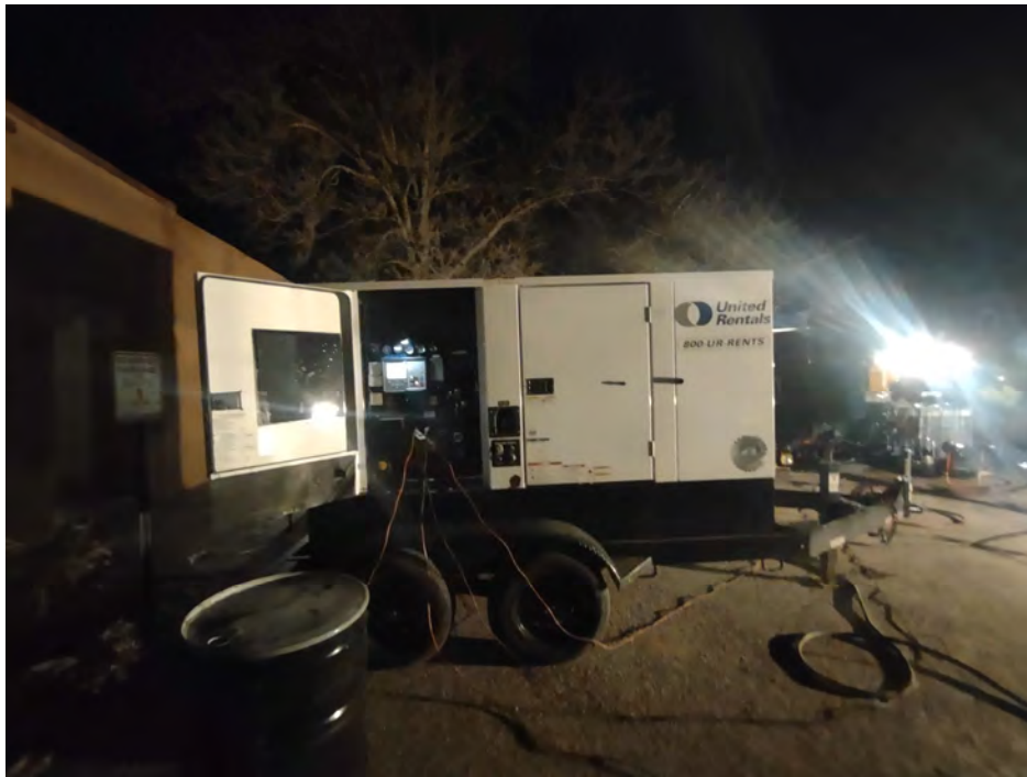
Trailer-Mounted MultiQuip 150 KVA Generator
