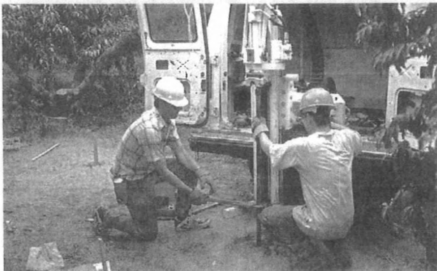
Nearly 3,000 feet of continuous soil cores were obtained between July and October 1997 using the Geoprobe direct-push drilling method. This method allowed for complete recovery of undisturbed cores throughout the 52-foot deep vadose zone. Above, UC Davis vadose zone hydrology professor Jan Hopmans (left) and Fresno State geology undergraduate Anthony Cole operate the coring equipment.
