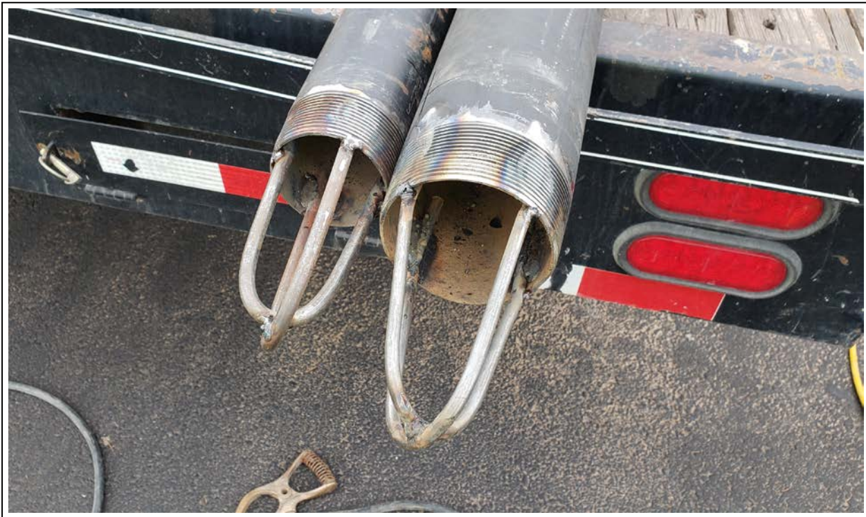
48. Dummies with welded loops for lifting with rig cables
