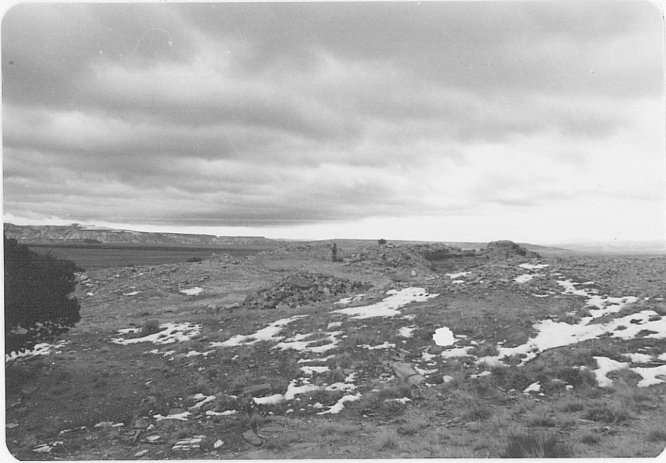
Photo (e) Looking eastward near north section line showing stripped area up to 16' deep in limestone; workings extend for about 400' into background; note person at left of center for scale.
