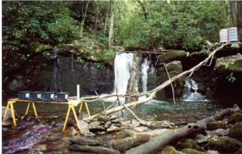
Figure 3. Sams Creek Potassium Permanganate station in operation, GRSM.
