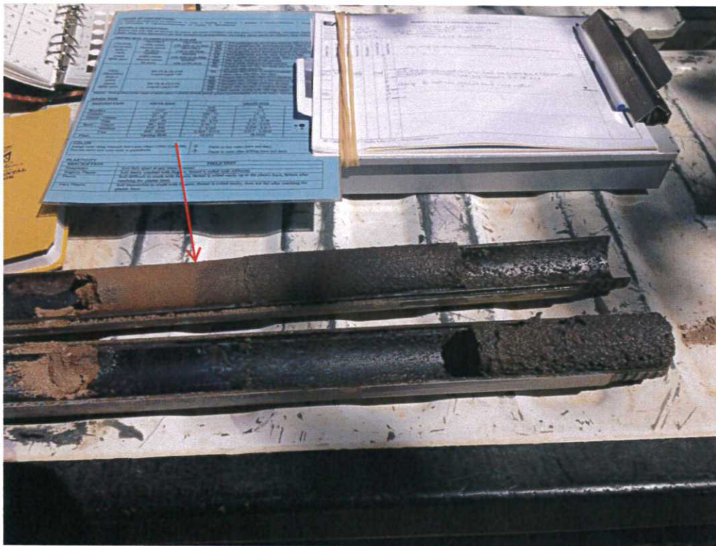
Photograph No. 6 Well MW-1 drill core showing petroleum contamination at groundwater interface.
