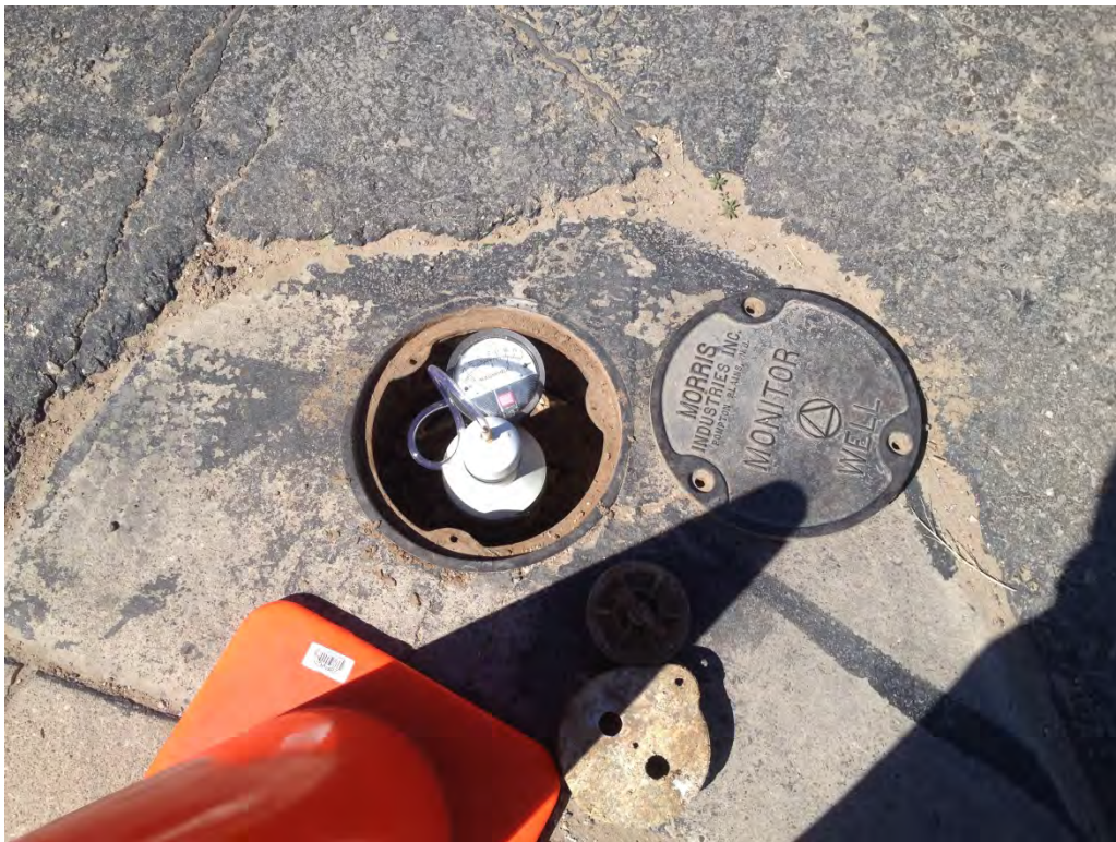
Photo 6: Walstad observation well setup with 2-inch Magnahelic gauge
