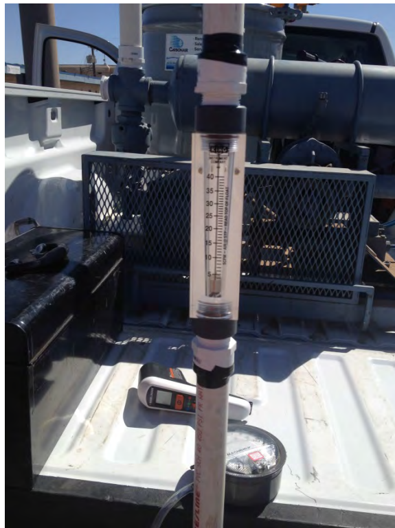
Photo 2: Walstad SVE pretest showing rotameter flow measurement device
