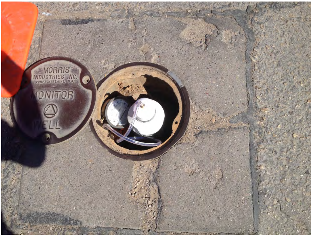
Photo 5: Walstad observation well setup with 1-inch Magnahelic gauge
