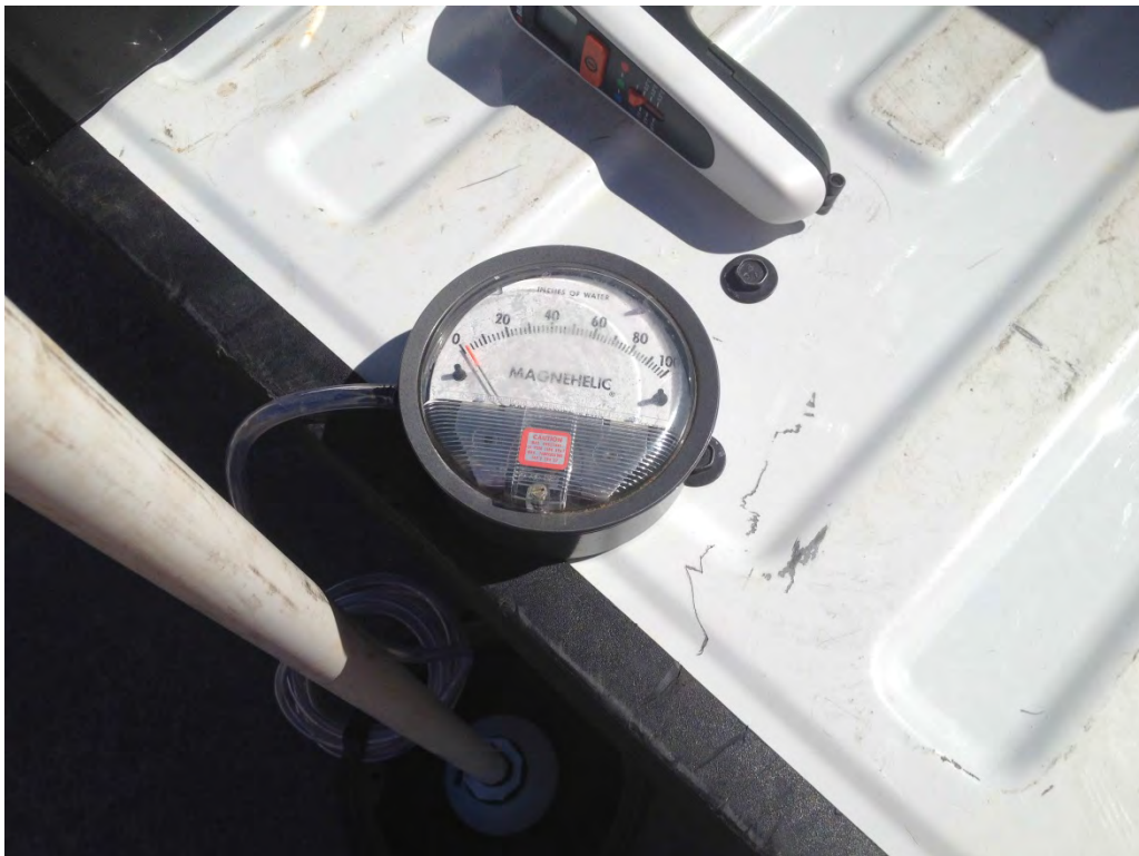
Photo 4: 100-inch H 2 O Magnahelic gauge for production well vacuum measurement
