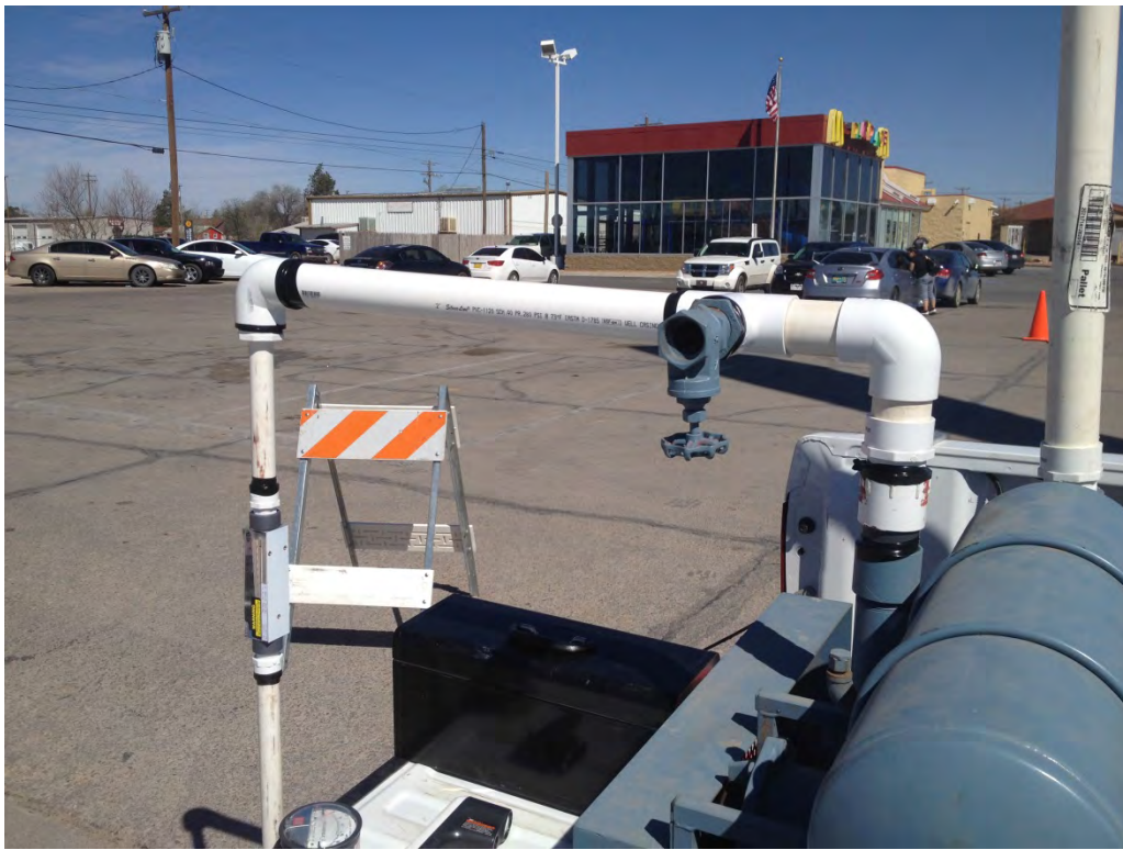
Photo 1: Walstad SVE pretest setup showing rotameter and flow control
