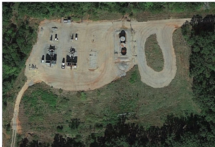
Figure 2: Typical gathering station shown in satellite imagery. Like many compressor stations, the station is not surrounded by a fence, but its boundary is clearly defined by a gravel pad.
