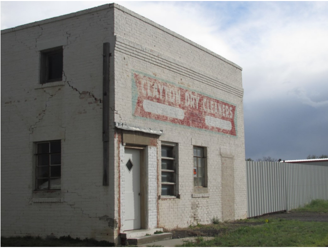
PCE, a chlorinated solvent, is still used at many dry cleaning facilities in the U.S. Some 60 sites on New Mexico's Orphan Site List, including this former operation in Clayton, have documented chlorinated solvent contamination, and because these fluids are heavier than water, they can penetrate deep into an aquifer.
