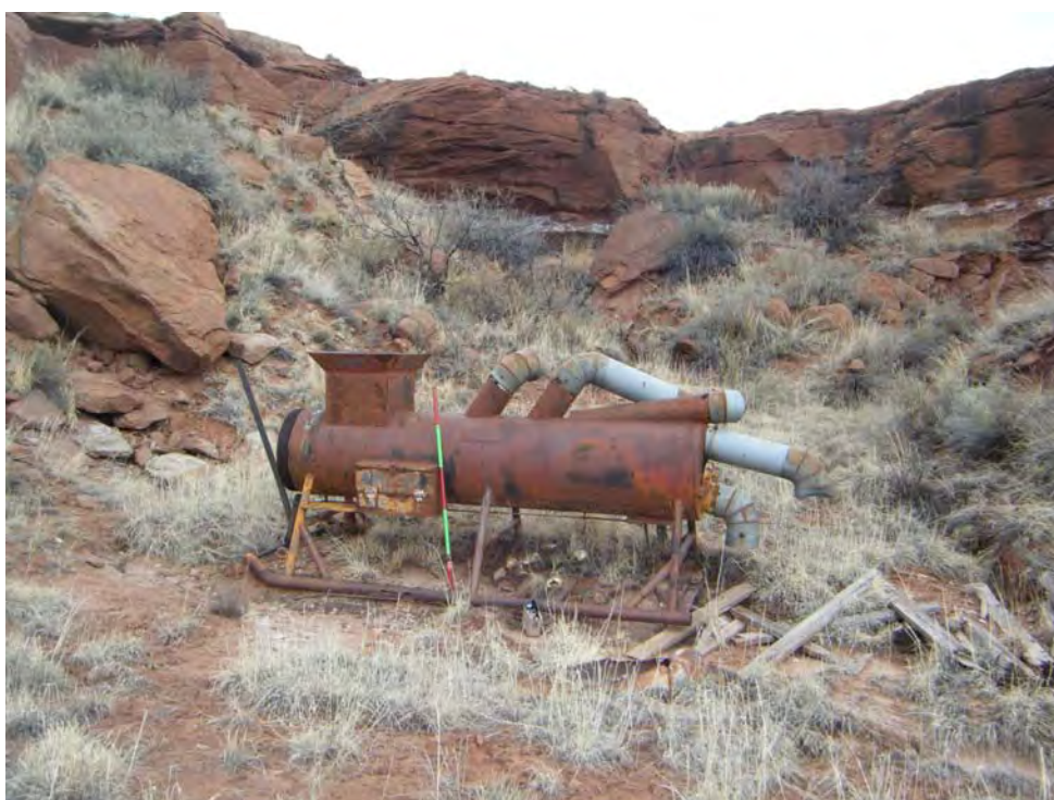
Photo 10-An ore sorter (according to Anderson, 1980) found onsite (Equip-2).
