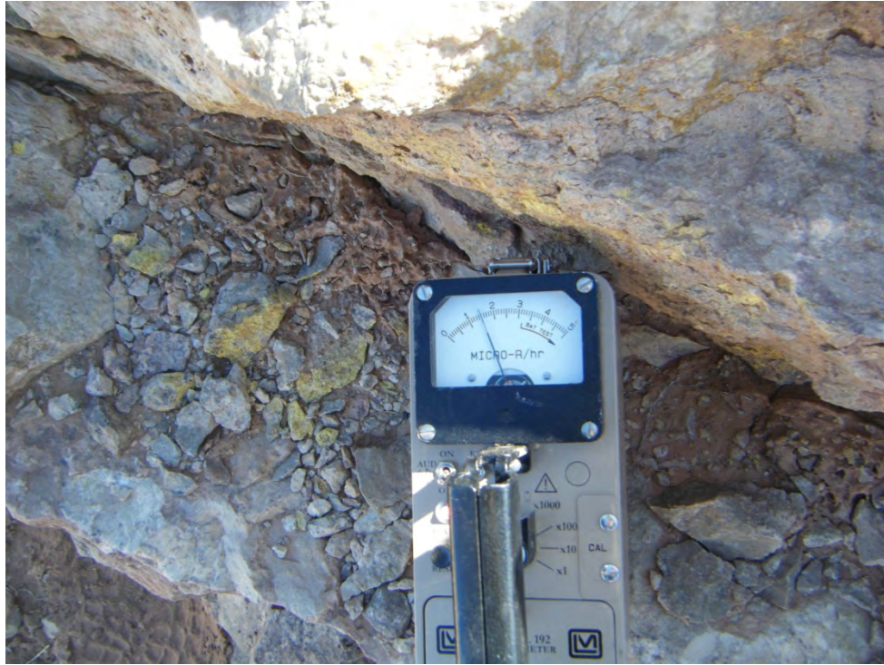
Photo 7-Radiation survey point 3 (1600 \mu R/hr at contact).
