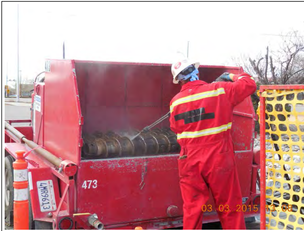
6. Decontamination of auger flights.
