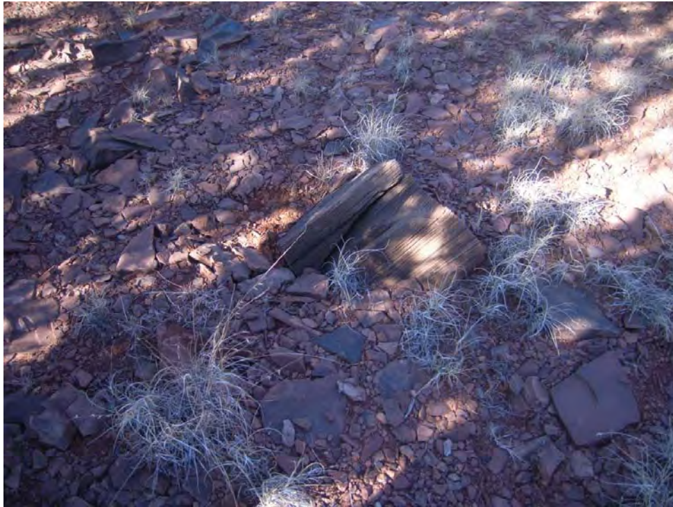
Photo 15 – Sandstone rock (rad-5) with radiation reading of 120 \mu R/hr.
