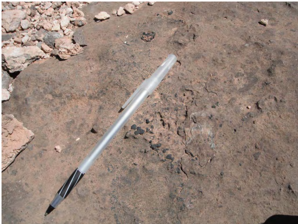
Photo 8-Closeup of rock at Rad-6. High radiation levels were found near the small, black inclusions in this rock.
