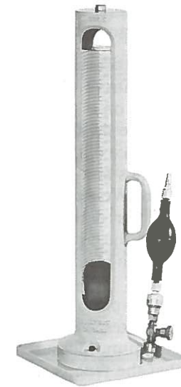
Fig. 13-3. Apparatus for determining soil bulk density in place by the rubber-balloon technique.
