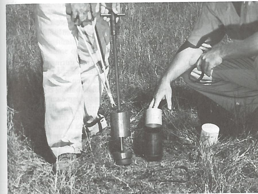
Fig. 13-1. Typical double-cylinder, hammer-driven core sampler, for obtaining soil samples for bulk density.
