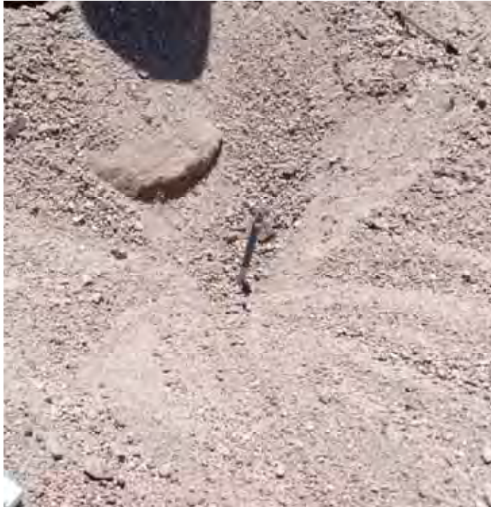
D3-3: Photographic reference for indicator 1.6. Photograph of 7 inch hole excavated in-channel. There is a complete lack of soil structure and moisture. Assessment unit is representative of channel bottom characteristics. Note dry mineral, sand sediments within channel.
