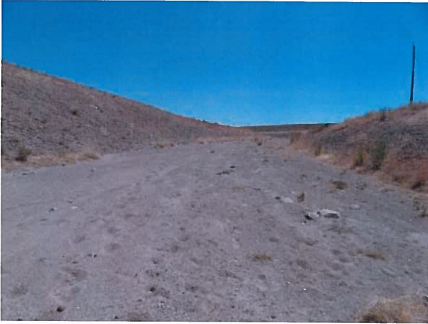
C5-1: Photographic reference for indicators 1.1 through 1.6. Indicator 1.6 scored as 2 – few rooted plants in the streambed. Lack of rooted plants is likely the result of the flow regime and granular bed material present rather than persistence of flow. No water or biotic indicators of water observed.
