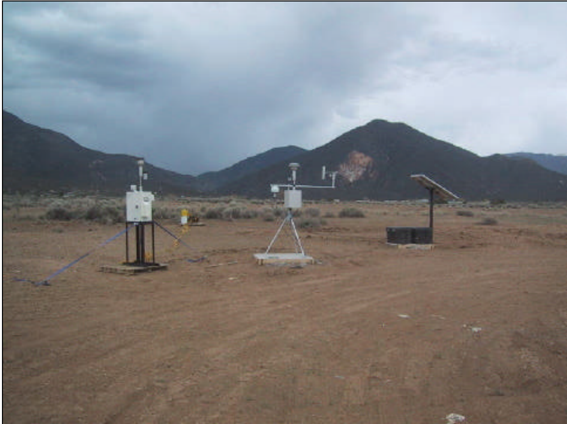
Figure 2. Metals Sampler Set Up (Partisol on left, EBAM in middle, solar array on right, generator in back)
