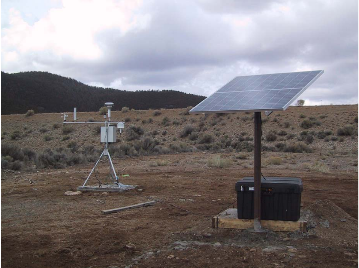
Figure 3. Photo of EBAM monitor and solar power system
