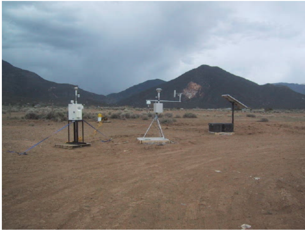
Figure 1. Metals Sampler alongside PM10 Monitor
