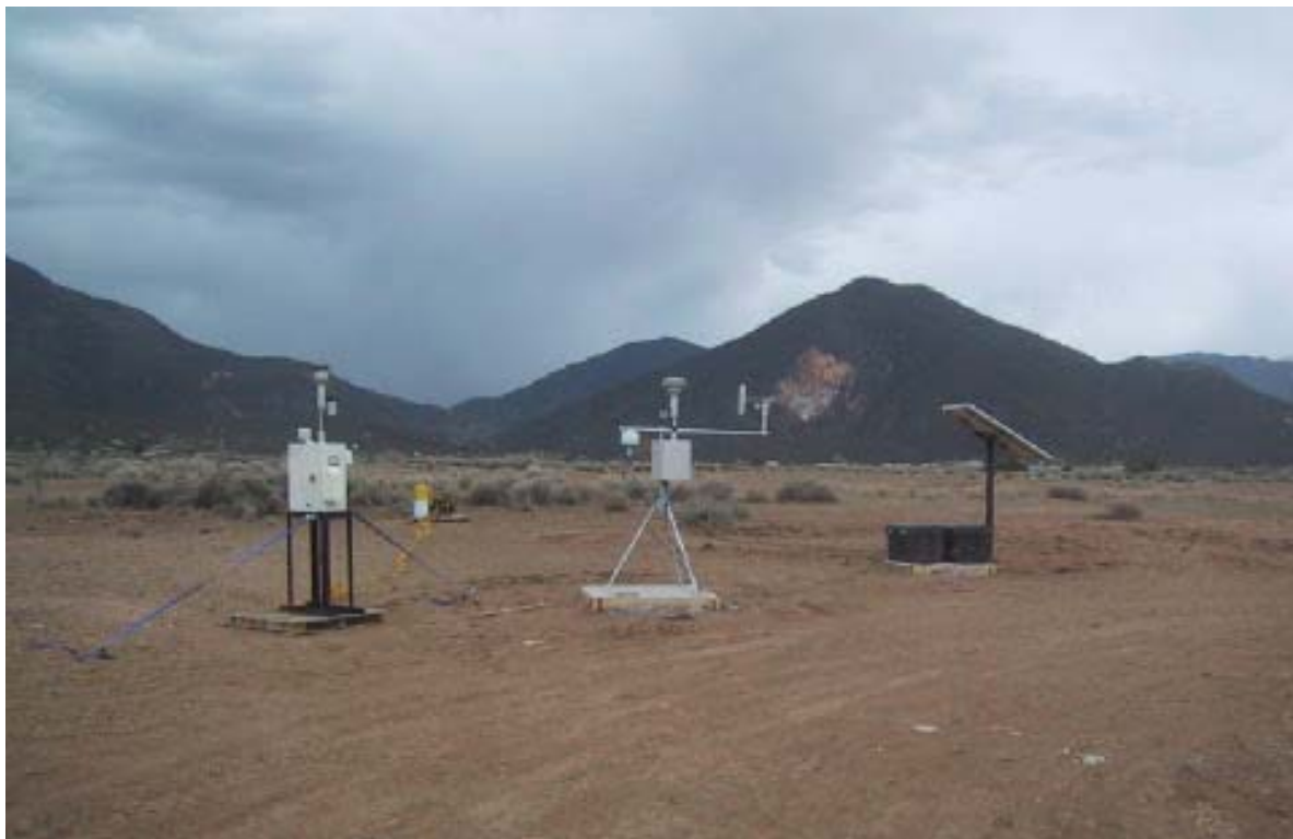
Figure 5. Metals sampler set up alongside EBAM PM10 monitor
