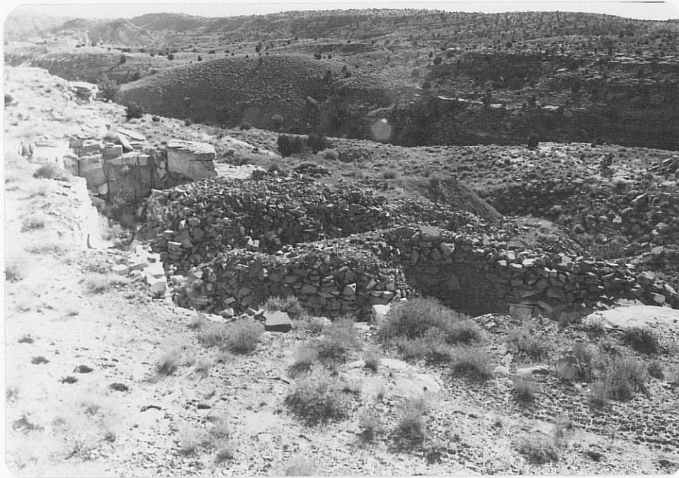
Photo (f) Looking SW at pit to the west of the workings in photo (c). Location is still in the S-SE corner of the VCA Plot #7. Note stacking of waste rock. Depth of trenching is 5' on left side of photo.
